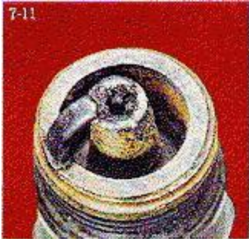
Pre-ignition (melting of the center electrode)
