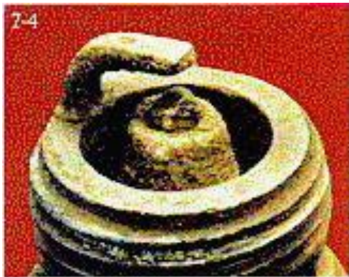
Worn (normal electrode erosion)
