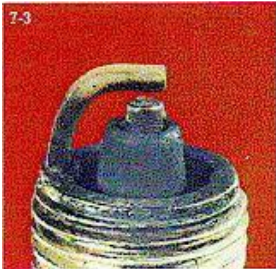
Carbon fouled plug ( Dry black appearance ).
