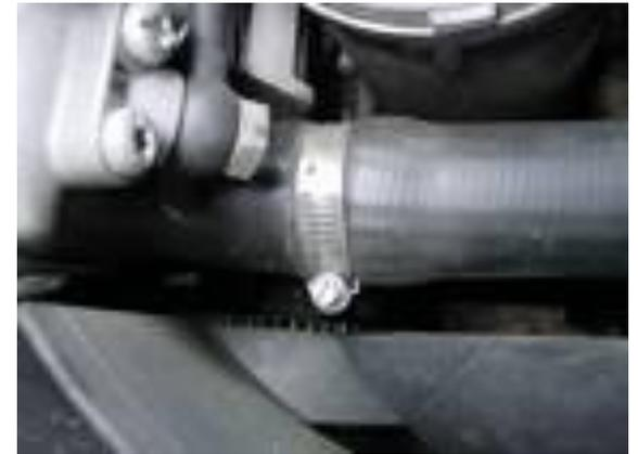
Lower radiator hose draws the coolant into the engine, from the radiator and is attached to the water pump. (sometimes a spring is inserted in order to prevent collapsing)
